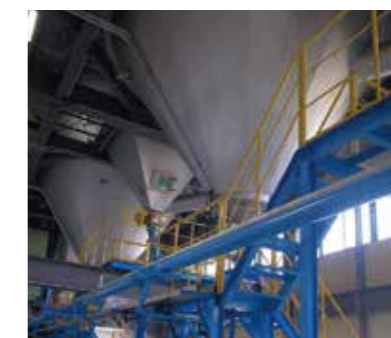
Atomization mode: Rotary atomizer Drying chamber diameter: φ5000 mm Liquid material processing capacity: 350 kg/h
