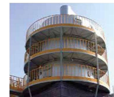
Atomization mode: Pressure nozzle Drying chamber diameter: φ4800 mm Water evaporation capacity: 1200 kg/h
